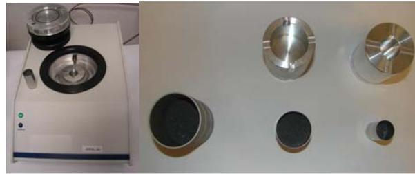
**Figure 2:** A typical helium pycnometer is shown on the left. The picture on the right shows three different cup sizes that may be used in this pycnometer for different sized parts
